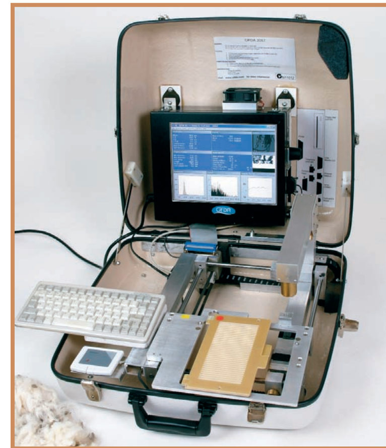
The OFDA 2000 is portable and meant for use in the field, for example, as animals are being sheared. The data screen shots at right are from the OFDA 2000.
